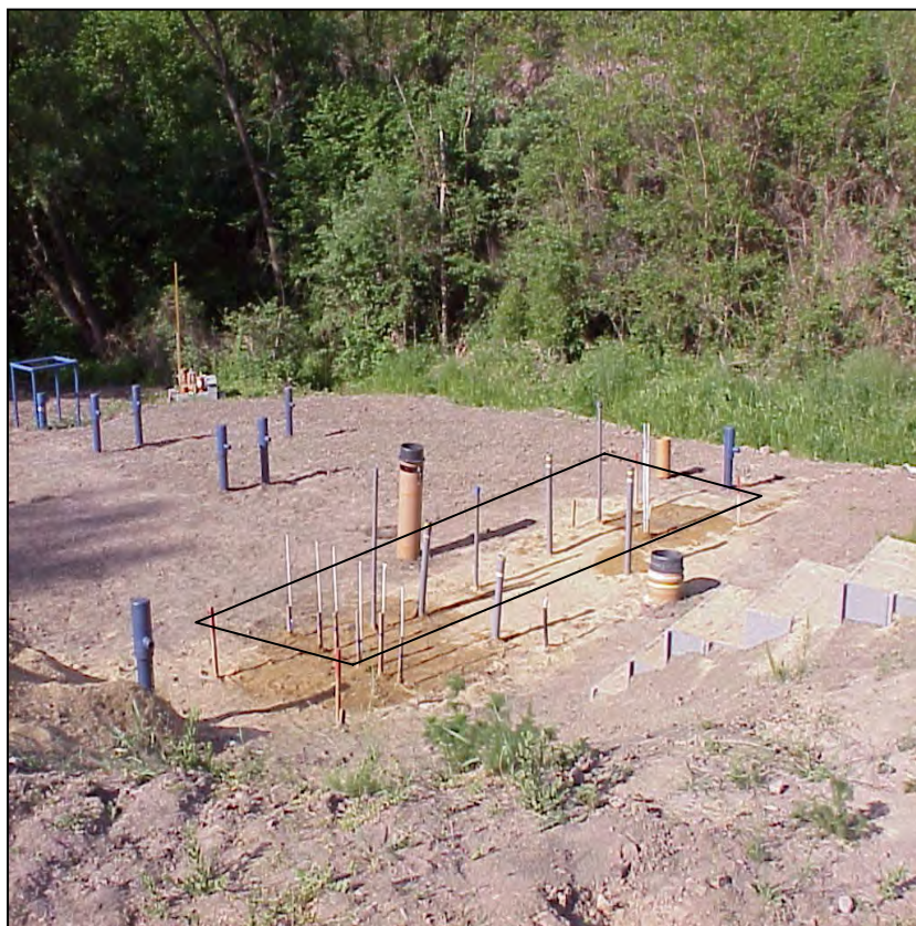
Fig. 14: Position of PRB with monitoring wells
